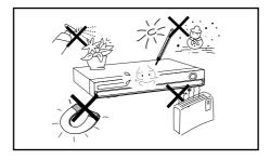
Protect the player from moisture (i.e. vases) , and excess heat (e.g.fireplace) or equipment creating strong magnetic or electric fields (i.e.speakers...). Disconnect the power cable from the AC supply if the player malfunctions. Your player is not intended for industrial use.
